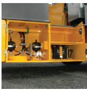
Compartments for operator tool box, lubricant storage, centralized greasing, brake accumulators and batteries
