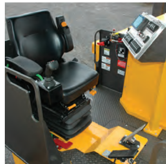
Comfortable swivel hydraulic suspension seat, dual armrests and joy-stick control
