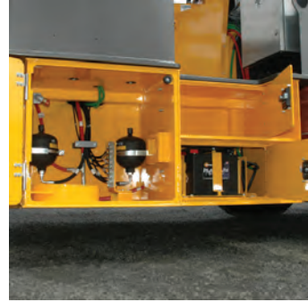
Compartments for operator tool box, lubricant storage, centralized greasing, brake accumulators and batteries
