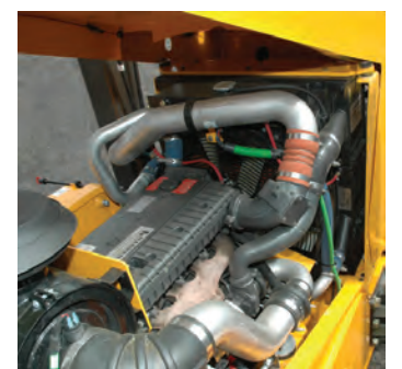
Hot and cold sides designed for additional safety
