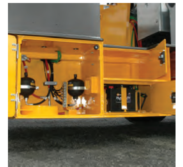
Compartments for operator tool box, lubricant storage, centralized greasing, brake accumulators and batteries
