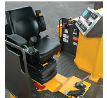
Comfortable swivel hydraulic suspension seat, dual armrests and joy-stick control
